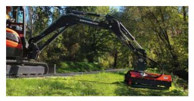
Hydraulic system for chopper with additional pump (22 lt/min)
