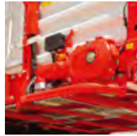
2-speed motor for scraper floor
