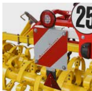
Warning signs and lighting
