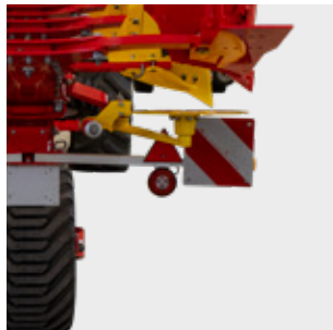
Warning signs and lighting
